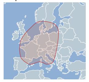
The footprint is the reception area on earth which a satellite covers with its transmission beam (spot) and in which satellite reception is possible. The transmission power is at its highest in the centre of this spot, and it becomes progressively weaker towards the edges.
